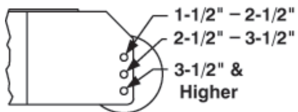
Height of cut ranges for roller adjustment
