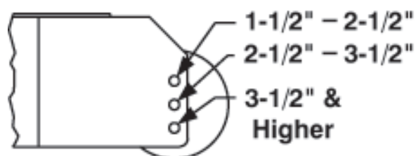
Height of cut ranges for roller adjustment
