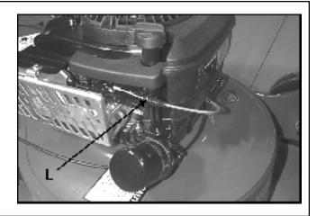
8. BRAKE CABLE - Secure the brake cable to the upper left handle with a 1/4-20 X 5/8" thread-forming bolt. Attach the eye of the cable wire to the "HOLD TO RUN" control arm at K with a 5/16 X 1/2" shoulder bolt, two washers and a locknut. Place both washers next to the bolt head. Route the brake cable under the handle assembly.
