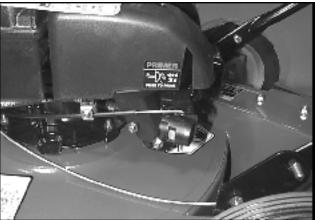
COMPLETED THROTTLE CABLE ASSEMBLY TO ENGINE
