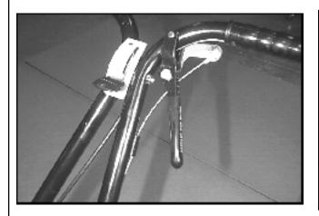
THROTTLE CLAMPED FOR ASSEMBLY TO HANDLE
