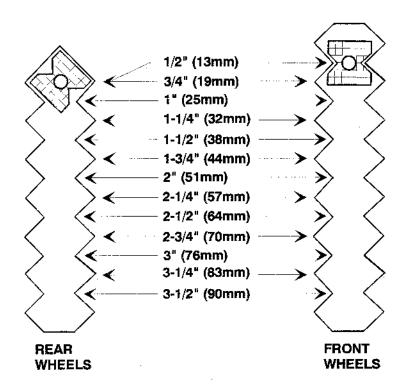
Wheel nut positions for 1/2" (13mm) cutting height. The rear wheel adjustment position is the same for 1/2" (13mm) and 3/4" (19mm) cutting heights. The setting shown above illustrates the 45° rotation of the adjustment nut between adjacent adjustment positions.
