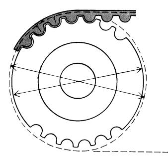
2228001 Sprocket Round Tooth Profile You can use both Round Tooth Belts and Square Tooth Belts on this Timing Sprocket.
