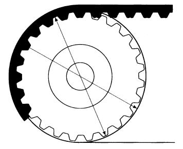
2720174 Sprocket Square Tooth Profile Use Square Tooth Belts only on this Timing Sprocket.
