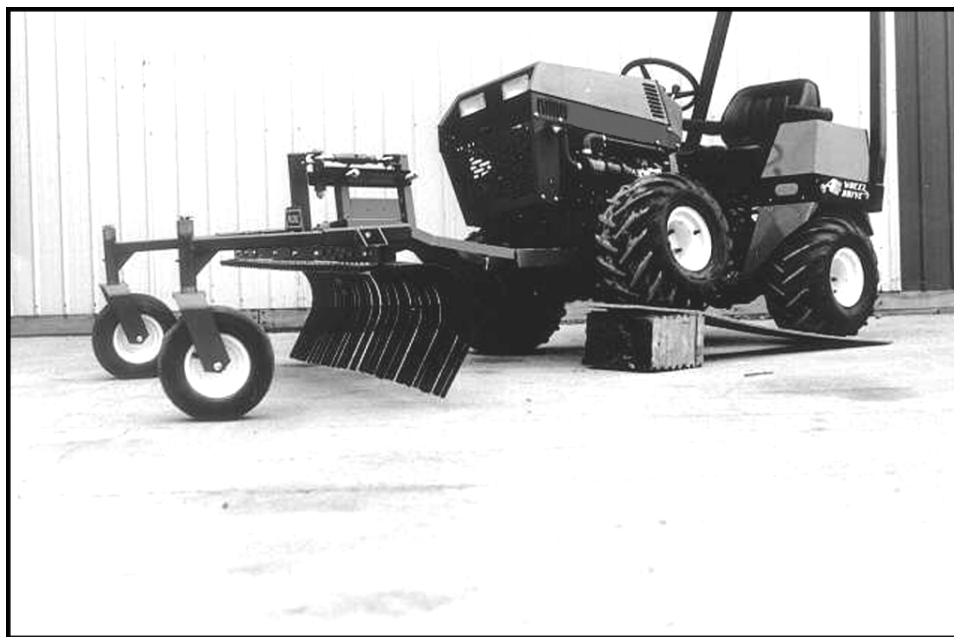
Spring loaded (factory set) for self leveling... independent of tractor angle.
