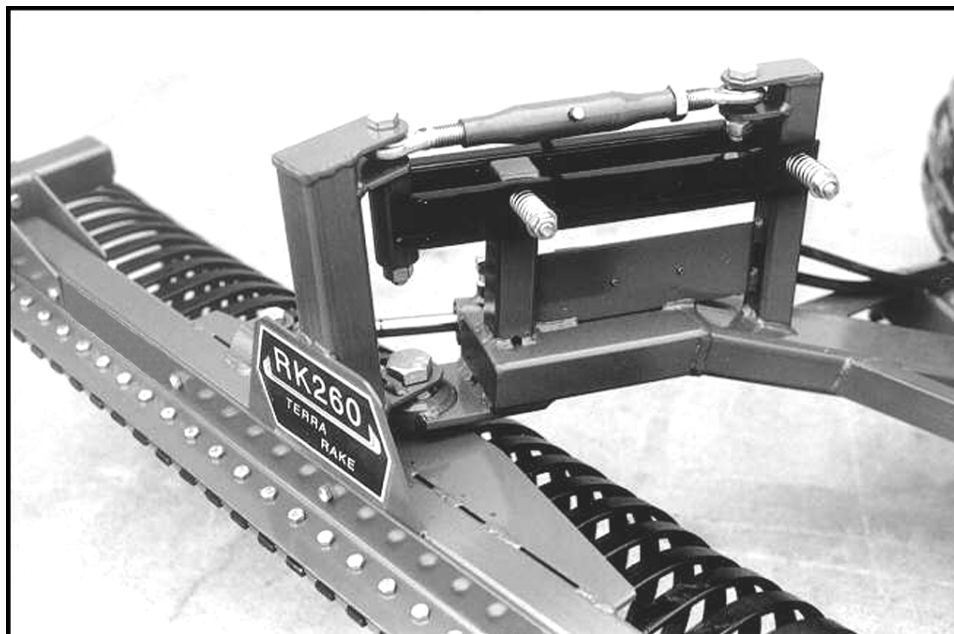
Top Link...provides fine tuning for depth adjustment
