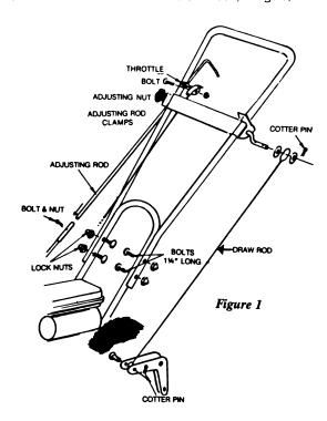
REFER TO PARTS EXPLOSION AND ILLUSTRATION AND ASSEMBLY YOUR PRO MODEL EDGER AS FOLLOWS:
