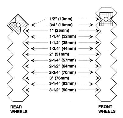
Wheel nut positions for 1/2" (13mm) cutting height. The rear wheel adjustment position is the same for 1/2" (13mm) and 3/4" (19mm) cutting heights. The setting shown above illustrates the  $45^{\circ}$  rotation of the adjustment nut between adjacent adjustment positions.
