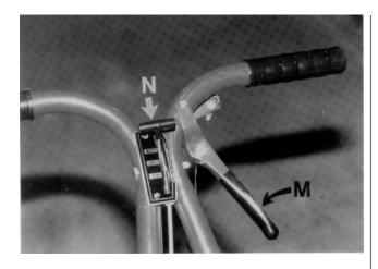
**HOLD TO RUN LEVER M-** Hold to handle bar to operate mower. Release lever to stop engine.
