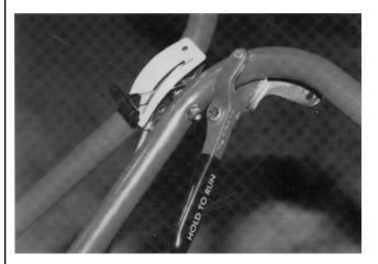
THROTTLE CLAMPED FOR ASSEMBLY TO HANDLE
