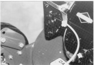
COMPLETED THROTTLE CABLE ASSEMBLY TO ENGINE
