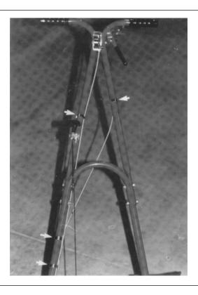
12. Attach the discharge chute to the mower housing with two 1/2-24 whizlock bolts and nuts.
