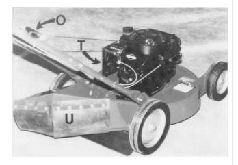
**RECOIL STARTER 0** - Pull and release to start engine.
