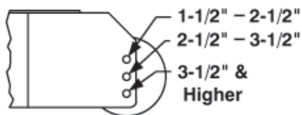
Height of cut ranges for roller adjustment
