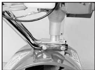
Picture 1 ... Note how the engine doesn't sit all the way down on the transmission.
