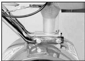
Picture 2 ... Note how the engine sits all the way down on the transmission.
