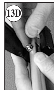
Fully tighten nuts and bolts installed in Step 9 located underneath handle brace.
