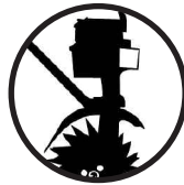
CAUTION: WHEN ASSEMBLING THE HANDLES, MAKE SURE FUEL TANK FACES AWAY FROM OPERATOR. THIS IS THE REAR OF THE TILLER, REFER TO ASSEMBLY INSTRUCTION ON PAGE 7.
