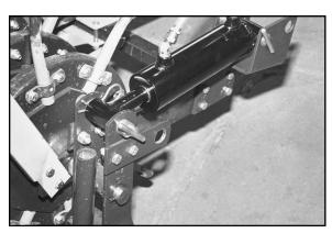
FIGURE 3 (For Tractors With 1500 p.s.i. Hydraulics) 1. Rear Hole Position on Pivot Bracket
