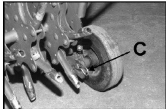
Lift up on the aerator handle so the tines are off the ground. With the tines off the ground, push the aerator through the gate on the front drum. Once on the other side of the gate, reinstall the wheels.
