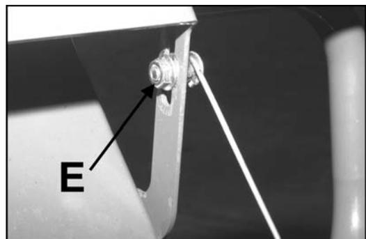
**CHECKING THE THROTTLE CABLE-** The throttle cable is adjusted prior to shipping; however, it should be checked before the unit is put into service. The throttle control should freely move in a full range of motion forward and backward. If necessary, the throttle cable can be adjusted as follows:
