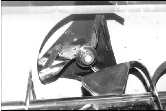
Photo 1 BLOWER SHEAR BOLT
