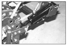
FIGURE 2 (For Tractors With 700 p.s.i. Hydraulics) 1. Cylinder Mounting Bracket
