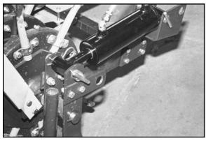
FIGURE 3 (For Tractors With 1500 p.s.i. Hydraulics) 1. Rear Hole Position on Pivot Bracket
