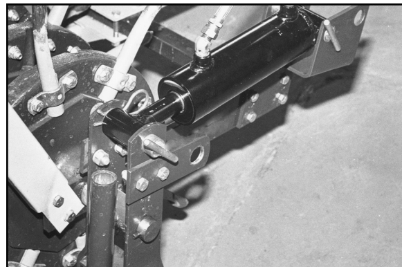
FIGURE 3 (For Tractors With 1500 p.s.i. Hydraulics) 1. Rear Hole Position on Pivot Bracket 2. Wheel and Leg Assembly
