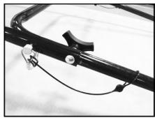
Mount the handle to the unit by placing the bottom ends of the handle over the pins at the top edge center of the chassis. Secure the handle with hairpins (from loose parts bag).
