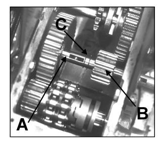
9. Assemble in reverse procedure. Apply 3M Scotch Grip 847 adhesive or equivalent to gear case cover before installation.
