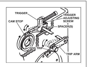
5. When all adjustments are made, re-tighten lock screw on trigger and run clutch through a few cycles. Determine if the clutch and brake system is working correctly, in not, additional adjustment will be required.
