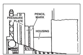
After stopping at the end of each cycle, check the pencil mark on the pressure plate. If the mark has slipped back 1/8" (3.2mm) or more, the brake and clutch clearance will have to be adjusted. Refer to the following sections on "Disassembly and Assembly"
