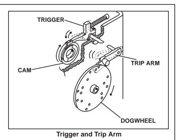
7. At the end of one revolution, the trigger slides into the notch of the cam locking it into position. The rollers are forced up the cam end incline, pulling the pressure plate into its braking position and locking the cutting blade in the up position.
