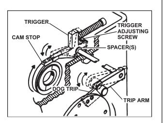
When all adjustments are made, re-tighten lock screw on trigger and run clutch through a few cycles. Determine if the clutch and brake system is working correctly, in not, additional adjustment will be required.
