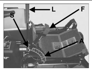
Lift and traction levers (operator's right side)
