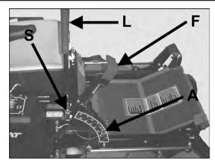
Lift and traction levers (operator's right side)
