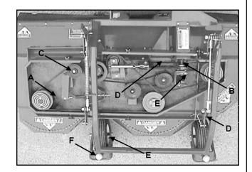
NOTE: It is necessary to remove the drive shaft shield and drive pulley shield to lubricate the drive line.
