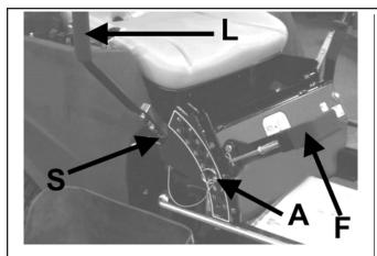
Lift and traction levers (operator's right side)
