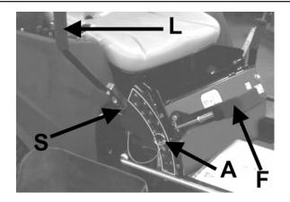
Lift and traction levers (operator's right side)
