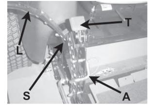
Lift and traction levers (operator's right side)
