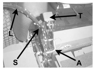
Lift and traction levers (operator's right side)
