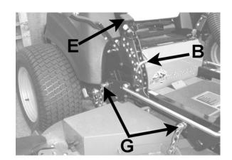
A 1/8" forward pitched deck provides the best horsepower.
