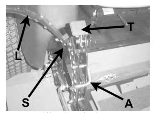
Lift and traction levers (operator's right side)
