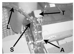
Lift and traction levers (operator's right side)
