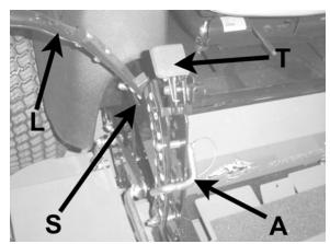
Lift and traction levers (operator's right side)
