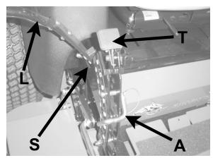
Lift and traction levers (operator's right side)
