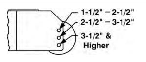
Height of cut ranges for roller adjustment
