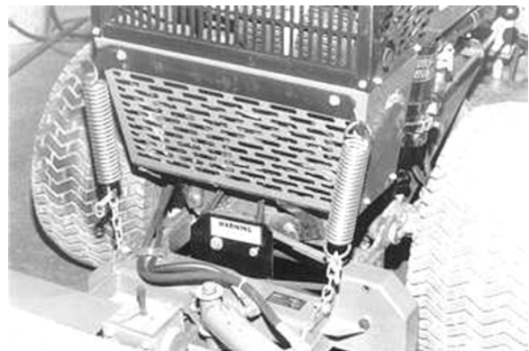
Photo 2 - Hose Clamp and Routing
