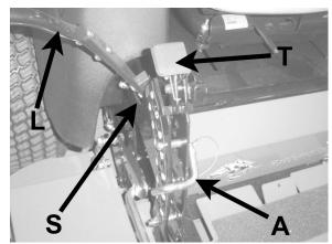
Lift and traction levers (operator's right side)
