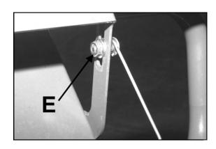
**NOTE:** Do not over tighten the chain. Excessive chain tension will reduce chain and bearing life. It can also lead to fatigue failure of the frame.
