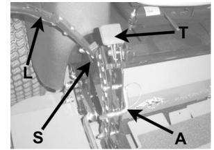
Lift and traction levers (operator's right side)
