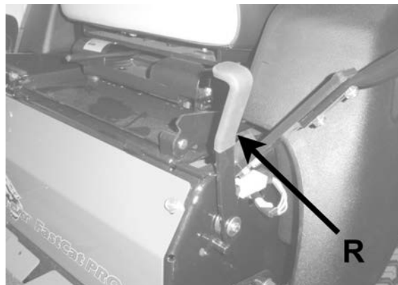
Parking brake in ON position (operator's left side)
