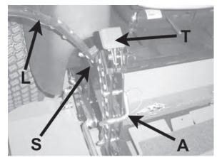
Lift and traction levers (operator's right side)
