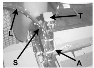
Lift and traction levers (operator's right side)
