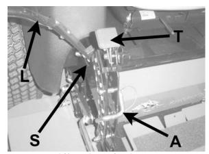
Lift and traction levers (operator's right side)
