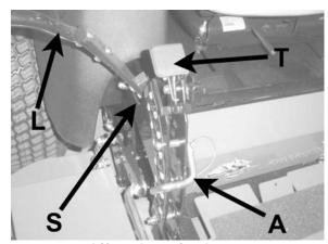
Lift and traction levers (operator's right side)
