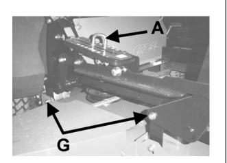
A level deck provides the best quality of cut. A 1/8" rearward pitched deck provides the best striping. A 1/8" forward pitched deck provides the best horsepower. Certain grass types and conditions may vary.
