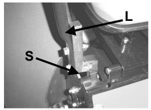
Lift and traction levers (operator's right side)
