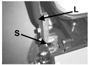
Lift and traction levers (operator's right side)
