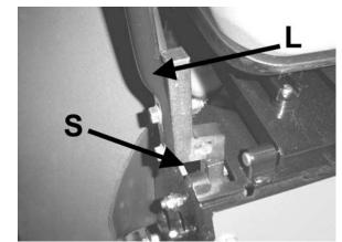
Lift and traction levers (operator's right side)
