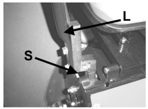
Lift and traction levers (operator's right side)
