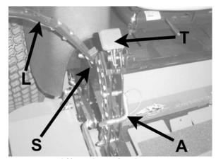
Lift and traction levers (operator's right side)
