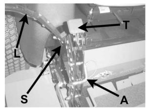
Lift and traction levers (operator's right side)
