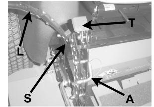
Lift and traction levers (operator's right side)
