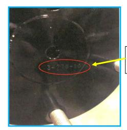
A stamped number as shown here indicates a good axle – not to be replaced.
