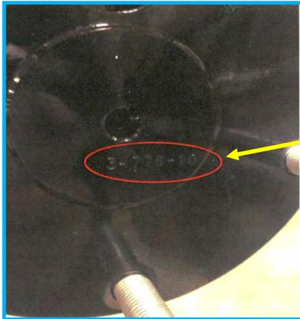
A stamped number as shown here indicates a good axle – not to be replaced.
